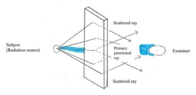
Radiation shielding material
